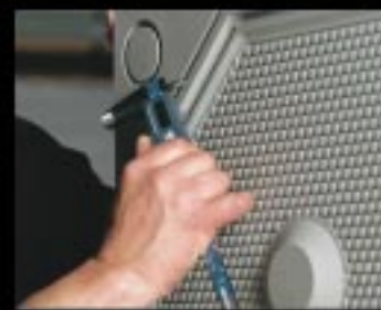
A Klinkau filter plate undergoes several quality inspections prior to shipping.
